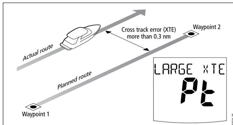
Cross track error (XTE) is the distance between the current position and a planned route. The SmartPilot receives the cross track error information
