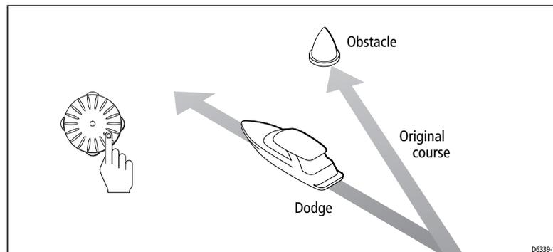
1. Select a course change in the appropriate direction. For example, turn the rotary control anti-clockwise for a dodge to port.
