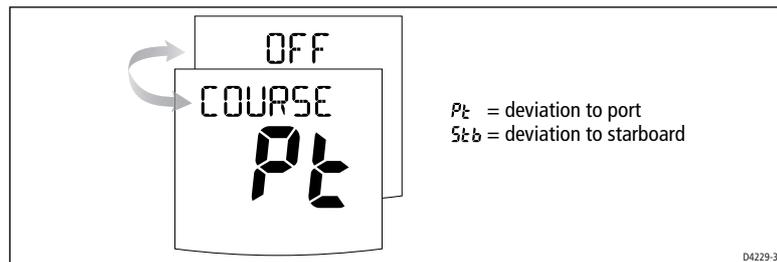
The SmartPilot warns you when you have been off course from the locked heading for longer than 20 seconds. It shows whether the deviation is to port or starboard.
