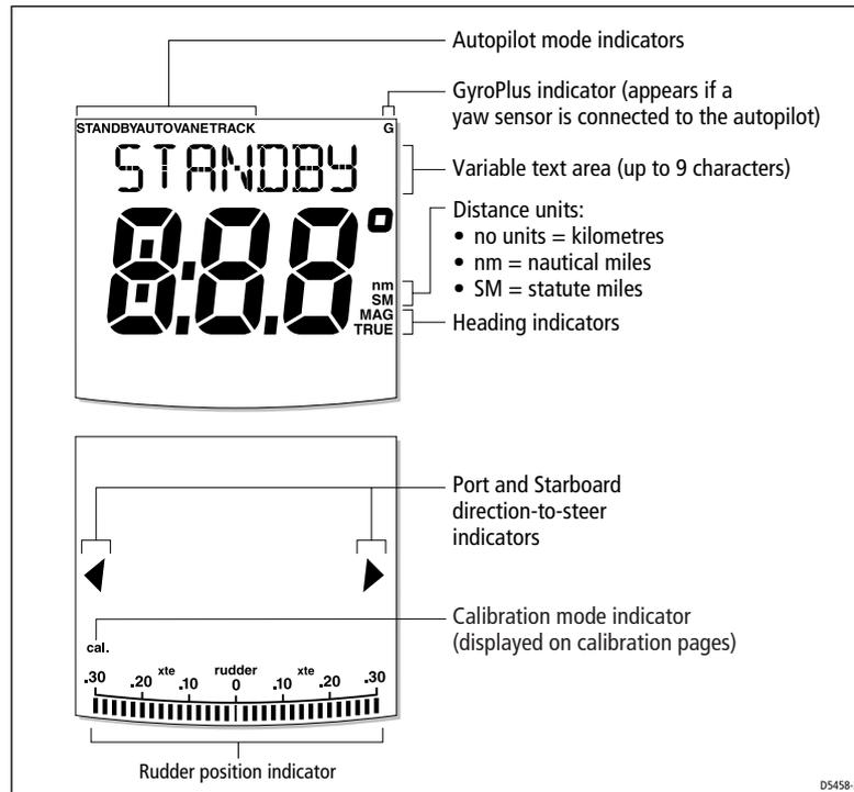
The bar graph at the bottom of the screen indicates the current position of the rudder, as measured by the rudder position sensor.
